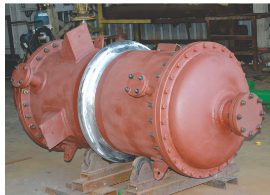
Heat Exchanger Re- Boiler
